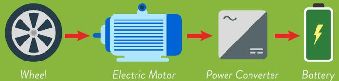
The flow of power during regenerative braking.
